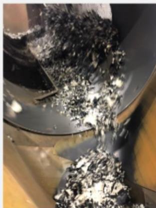
Grain bags are shredded and screened before washing...
